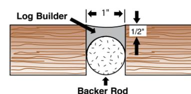
For joints 1" wide or more, the depth should be 3/8" to 1/2". The depth of joints less
